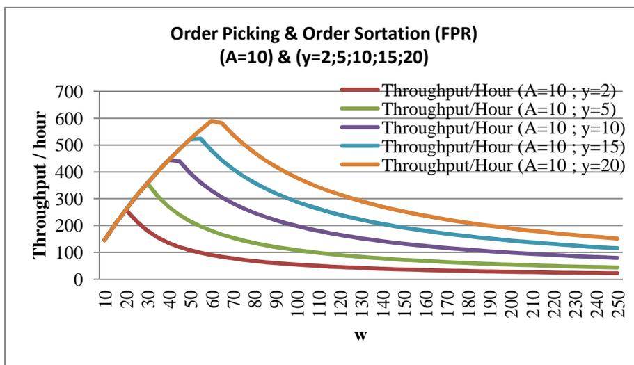
Figure 4: Hourly throughput rate of the system for (A=10) & (y=2;5;10;15;20)
