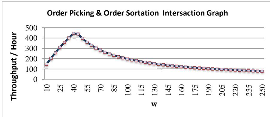
Figure 3: Changes in hourly throughput rate of the system for different wave size.
