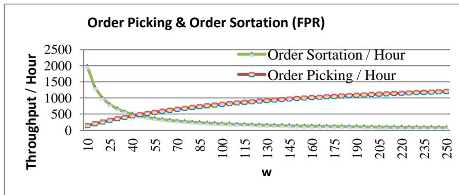
**Figure 2: Hourly throughput rate of order picking and order sortation operation**
